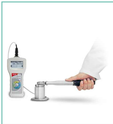
The way of checking torque wrenches
