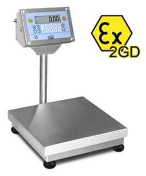
Fully stainless steel bench scales, for specific use in <u>ATEX</u> hazardous areas. Powered by a long lasting rechargeable battery which allows an easier installation directly where it's needed. These scales don't need a power supply socket in dangerous zone nor ATEX proof power supply cables. Provided with the ATEX declaration of conformity. Ex II 2G IIC T4 Gb X and Ex II 2D IIIC T197°C Db X protection.
