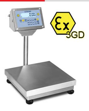
Fully stainless steel bench scales, for specific use in <u>ATEX</u> hazardous areas. Powered by a long lasting rechargeable battery which allows an easier installation directly where it's needed. These scales don't need a power supply socket in dangerous zone nor ATEX proof power supply cables. Provided with ATEX declaration of conformity. Ex II 3G IIC T6 Gc X and Ex II 3D IIIC T115°C Dc X.
