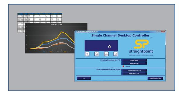
Windows based software package. DCP10M simply plugs into the spare port on the loadcell and connects to a Windows based PC, laptop or tablet.
