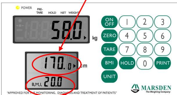
The automatic height measurement also enables the automatic calculation and display of the Body Mass Index (BMI) of the measured person.
