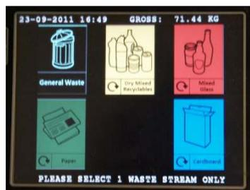
4. To select a waste type press and hold the corresponding waste image until a white outline is shown around the selected image.
