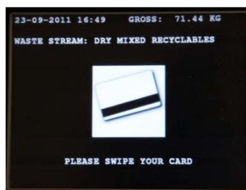
5. To finish the weighing transaction, simply swipe a card on the card reader. The indicator will show a confirmation of the transaction.
